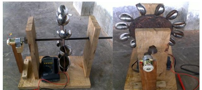
Fig.4: Manufactured pelton wheel (Front & Side view)
